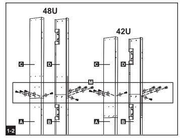
Insert the lower end of the left vertical section into the bottom section **E** as shown. Align the screw holes, insert four M5 x 10 mm screws and washers **M** and tighten securely. (Start all the screws before tightening.) Repeat this step for the right vertical section.
